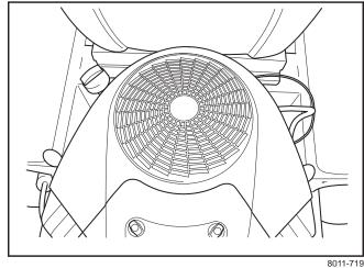
Check and clean the cooling air intake
