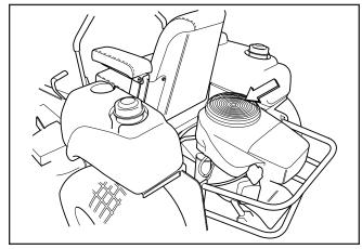
Check and clean the cooling air intake
