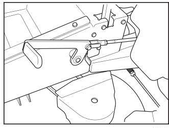
The parking brake in the disengaged position
